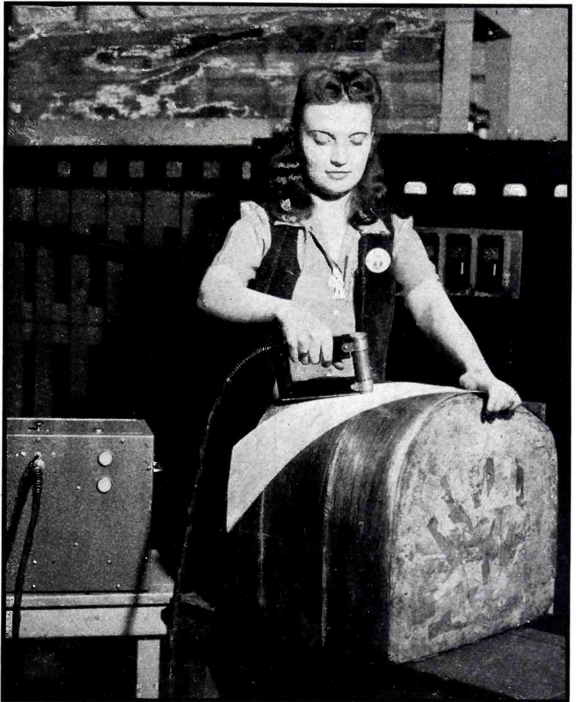
Using the special ironing-type r-f gun to smooth out and tack down layers of veneer on a mandrel, in much the same way that the wire stapler is ordinarily used
