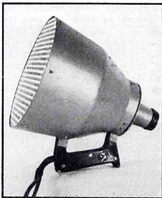
Electronic megaphone unit as made for U. S. Navy by Powers Electronic & Communication Co. It differs in some details from the equipment described in the text, but serves the same military purposes
