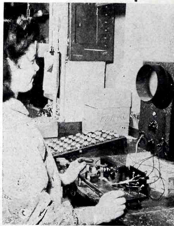
Production testing of potentiometers is accomplished by placing each control in a fixture that rotates the shaft and plots the resistance versus rotation on the screen of a cathode-ray tube
