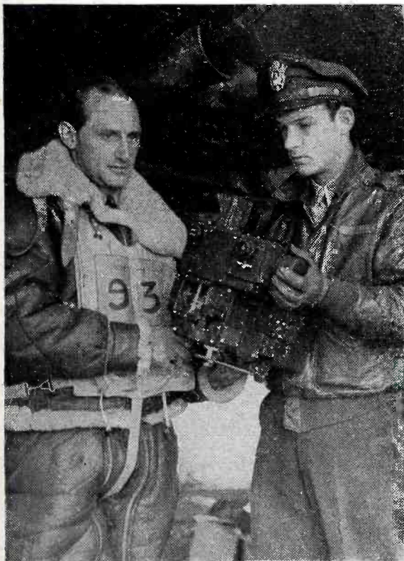
Shown here is the Sperry computing gun sight, a model of scientific precision, used on Flying Fortresses. The gun sight makes corrections for the factors such as plane and wind velocity which might otherwise cause a gunner to miss his mark
