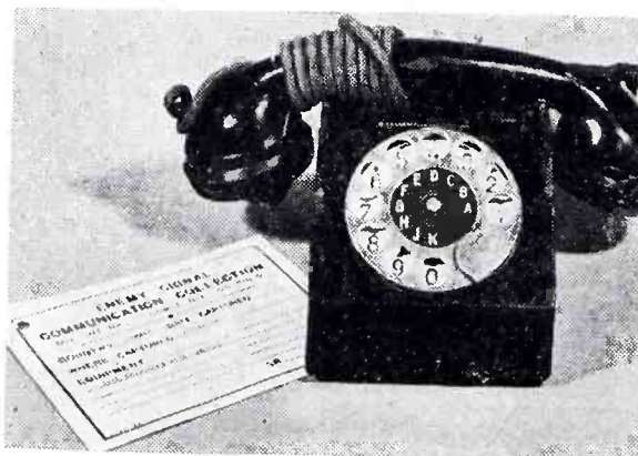
German dial type field telephone switch box for two lines, complete with hand set
