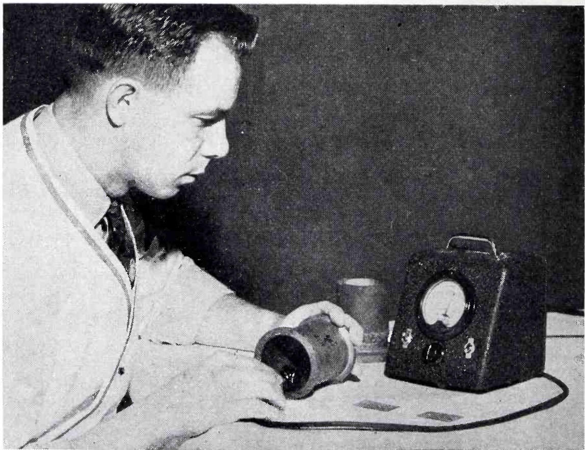
Measuring babbitt thickness of a bearing with a G-E reactance-type thickness gage
